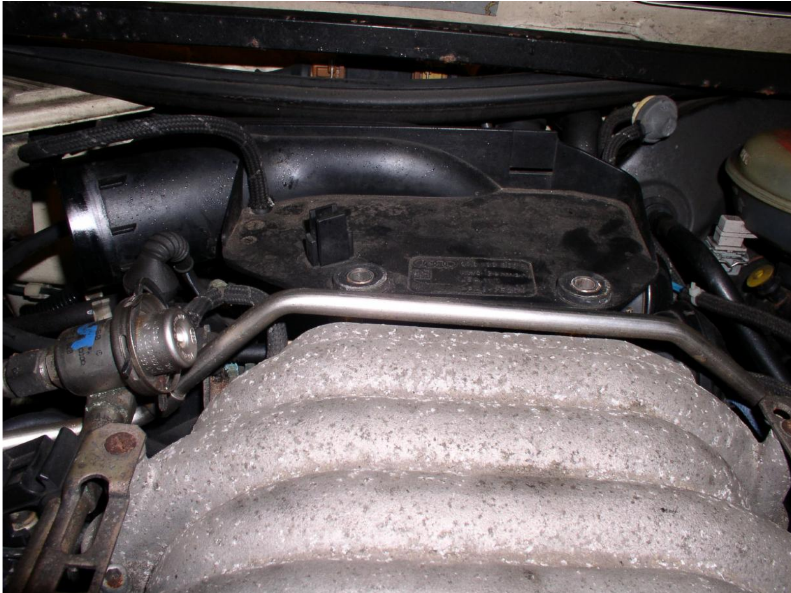
Close-up of the plenum top.
